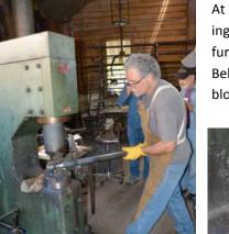
At left Joe's using the drawing dies on his hammer to further work the pipe.
